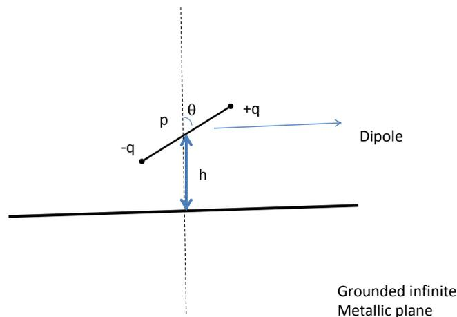
Figure 1: A dipole above a grounded infinite metallic plane.
